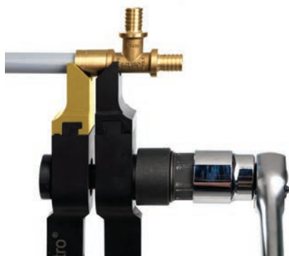
▲ Fig. 27: Use the tool to push the compression sleeve right up to the fitting collar.
