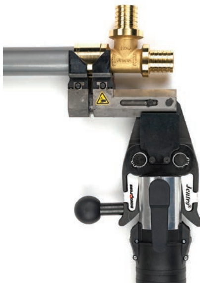
▲ Fig. 94: Operate the drive unit to push the compression sleeve right up to the fitting collar.
