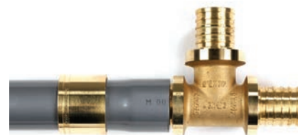
▲ Fig. 92: Push the fitting into the pipe. After a short period of time, the fitting has a tight fit in the pipe. (PEX has a larger "memory" effect than STABIL).
