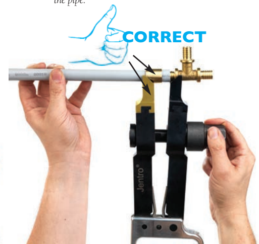
▲ Fig. 26: The yellow clamping head has a special shape on the inner side and it should always be pressed against the sleeve!
