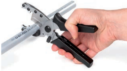
▲ Fig. 18: Cut the pipe to the requested length. Caution! Always cut the pipe in a square cut!
