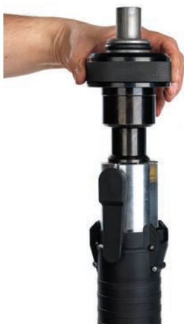
▲ Fig. 90: Mount the expander together with the nut (art. 15305).
