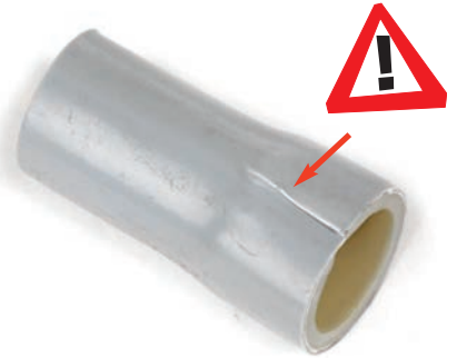
▲ Fig. 98: STABIL pipe cut off slantwise and ruptured during expansion. Cut off the pipe straight and expand again.
