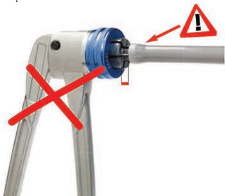
▲ Fig. 29: Pipe NOT until end of expander.
