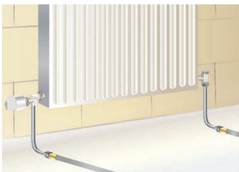
▲ Fig. 115: Connection with L ensembles twice at the bottom.
