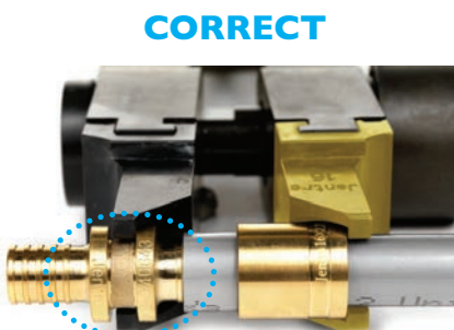
▲ Fig. 38: Black clamping head placed correctly.
