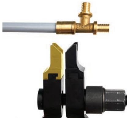
▲ Fig. 28: Turn the clamping jaws open again.
