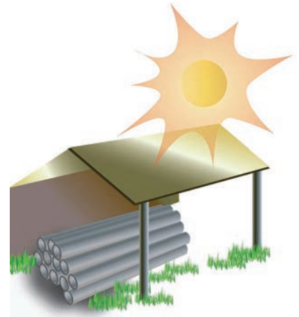
▲ Fig. 6: Protect pipes against U.V. radiation
