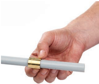
▲ Fig. 21: Push the compression sleeve over the pipe. The inside chamfer has to point to the end of the pipe.
