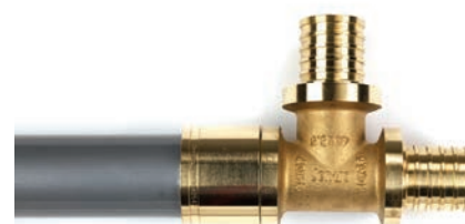
▲ Fig. 95: Compression joint ready. Sleeve right up to the flange edge.
