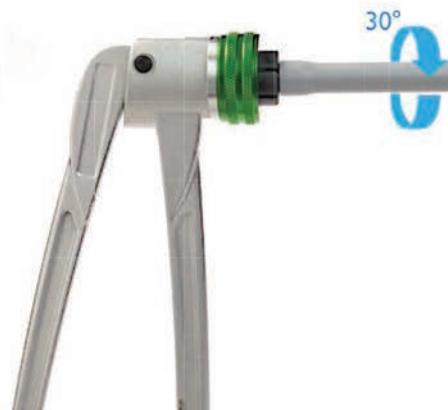
▲ Fig. 34: Expand STABIL pipe.
