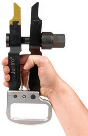
▲ Fig. 24: Caution: the clamping head behind the sleeve has a yellow chromed colour; use behind the flange edge the head with black colour!
